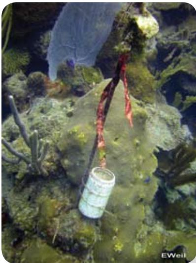
Figure 4.11 A sediment trap can be deployed to quantify the amount of silt and other particulate matter settling onto a reef. Photo: E.Weil
