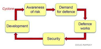
a larger cyclone event then occurs, or the wall does not protect the assets sufficiently, and there is demand for a larger and stronger wall. This cycle continues, with the amount of assets located in an area exposed to coastal hazards ever increasing. The root cause of the issue-that people are developing in an area exposed to coastal hazards-is not being addressed.
