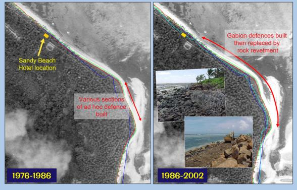
Over the subsequent decade, various gabion defenses were installed to protect sections of the road, with the length of the defense increasing over time. However, the gabion baskets quickly broke down, releasing volcanic rock that ended up covering the beach in front of the hotel. This resulted in a legal case brought by the hotel against Kosrae State asking for the rocks to be removed from the hotel beach.
