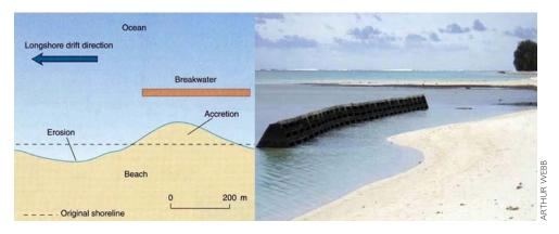
c. Breakwaters: Breakwaters are hard defenses placed in the sea, parallel to the shoreline, to break up wave energy before it reaches the shoreline. However, like other structures breakwaters also influence long-shore movement of beach sediment, with sediment often building up behind the structure at the expense of the beach areas on either side.
