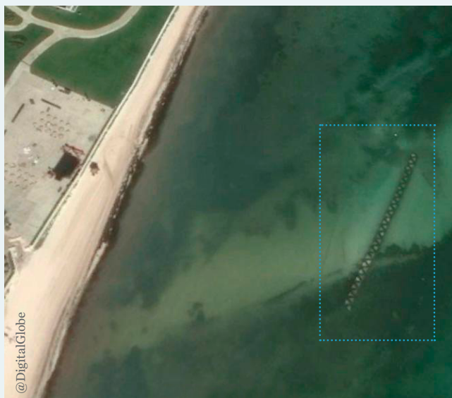
FIGURE 9 | WADs used in the construction of a submerged breakwater located in the Mexican Caribbean, specifically in Puerto Morelos, outside the protected area (Silva et al. 2016).
